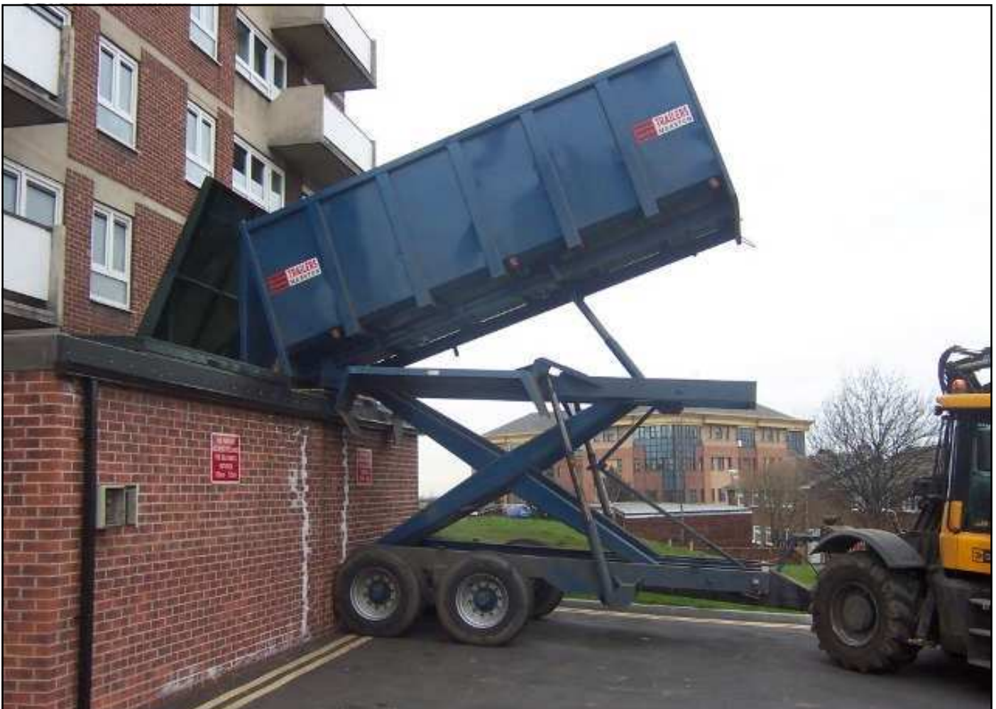
Above: Purpose built woodfuel storage bunkers with hydraulic lids. Fuel is delivered into the bunker using a high “scissor lift” fuel trailer.
